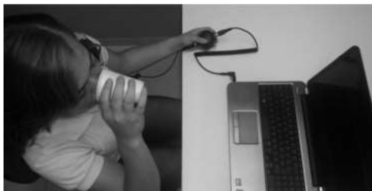
Figure 3. Image of the subject who drank 180 ml of water and pressed the release button of the microphone channel while recording the audio.
