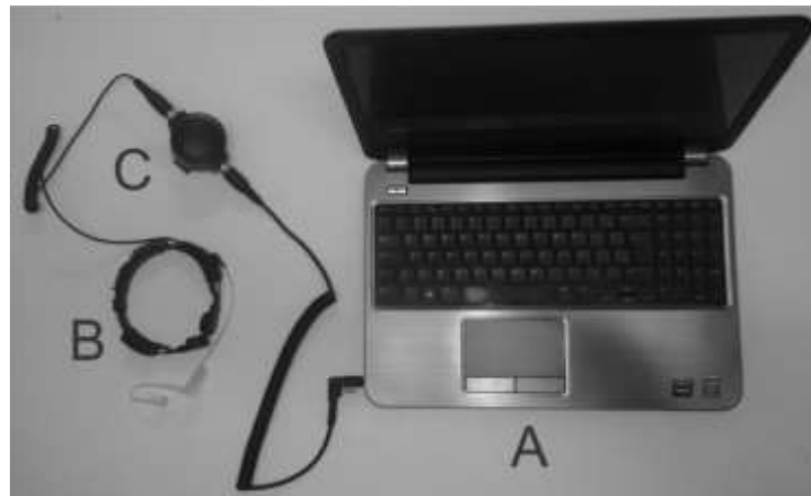
Figure 2. Image of the devices used in the experiment: in A, the laptop is used for the storage and processing of the signal; the element B is the throat microphone used for the acquisition of the audio produced during the swallowing of food; the element C is the microphone button that allows the release of the channel, allowing the recording to be made.
